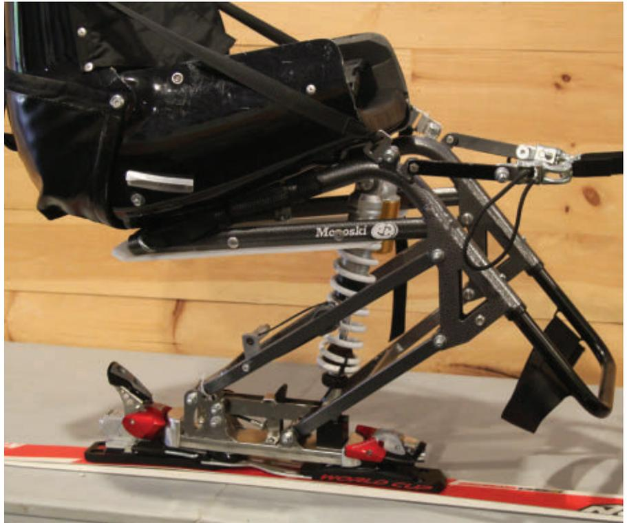
**Photo 1: The overall surface lift setup. The quick release hardware is positioned on both sides and within easy reach for the skier.**
